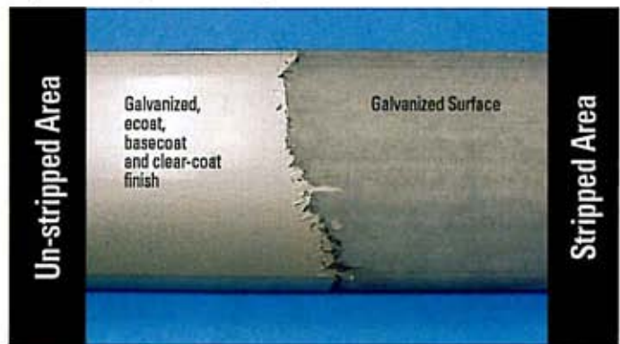
The layers of organic coating have been removed from half of this rail.
